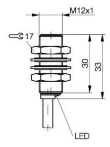
Inductive Sensors BES 516-325-E4-C-PU-03 M12x1 x 33 normally-open Sn=2mm shielded
